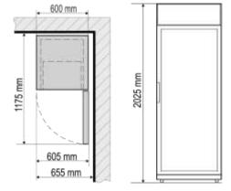
• The appliance must stand on a level surface and must not touch the wall. If necessary, regulate the height of the appliance by adjusting the levelling feet: by turning them clockwise – the front of the appliance rises, by turning them counter clockwise – it comes down. If the appliance is tilted slightly backward – the doors will close by themselves.
